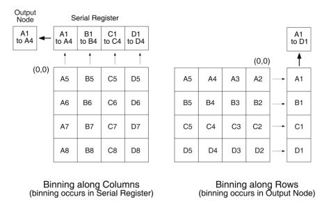
Figure 27. Binning and Array Orientation
